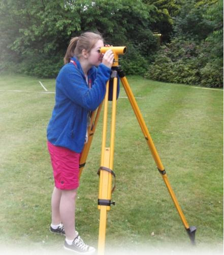
around the site. After recording the height of the land, we set about mapping the key features of the site such as the foliage covering a large portion of the site. Using the existing plans of the Science block and Sixth Form block, we measured the distance from the foliage boarder to one point on the Science block and another point from the Sixth Form block. This has enabled us to triangulate the position of the foliage in relation to the two blocks.
